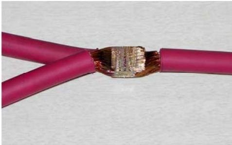
the oxides and surface films, creating a true metallurgical weld. There is no melting of materials. In addition to creating a very reliable bond, the process is
