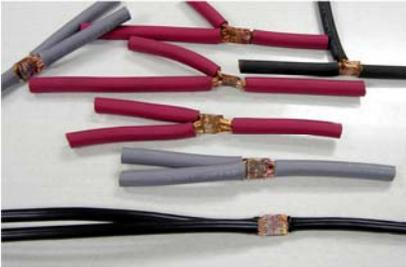
*comfortably weld wire bundles with cross-sectional areas of up to 100 square millimeters. This same unit also accommodates tinned or heavily oxidized wires that might otherwise stall the welding*
