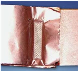
appropriate tooling, the Dual Head Spot Welder can weld non-ferrous sheet metal. In addition, it can weld up to 80 layers of foils, making it ideal for advanced battery and super capacitor applications.
