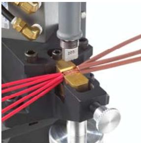
heavily oxidized. It does this without melting the wires or producing arcs, sparks, or fumes. In addition, the SpliceRite™ eliminates the insulation burnback, cooling
