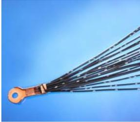
Sonobond equipment is used to weld stranded wire-to-wire and wire-to-terminal for applications such as electrical wire harnesses and bus bars. This metal welding technology is also used to weld the terminals of lithium-ion batteries, foil-
