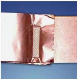
**Advanced battery and super capacitor applications** involving up to 80 layers of foils even if lightly tinned. The dual-head system can also weld 3 millimeter-thick, non-ferrous sheet metal when equipped with appropriate tooling.
