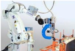
**Welding of larger metal parts,** such as those used in the automotive industry. The “C-frame” units virtually eliminate the problem of tips sticking to aluminum parts and can be equipped for use on large industrial robots.
