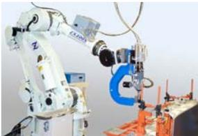
throat. The welders can also be operated by a robot arm.
